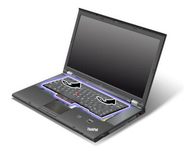
3. Push down the keyboard firmly and then slide the keyboard in the direction shown by the arrows.
